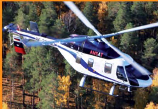
With the help of quick-detachable equipment, the Ansat, a light twin-engine multipurpose helicopter, can be quickly re-equipped to perform a wide range of tasks, including transportation of goods and passengers, surveillance, search and rescue, fire fighting and medevacs.
